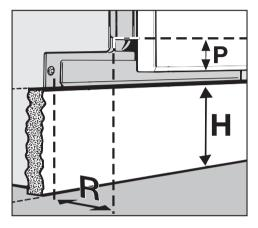
The height (**H**) of the plinth facia in front of the dishwasher depends on the plinth return (**R**) and how much the door front extends below the dishwasher door (**P**).
